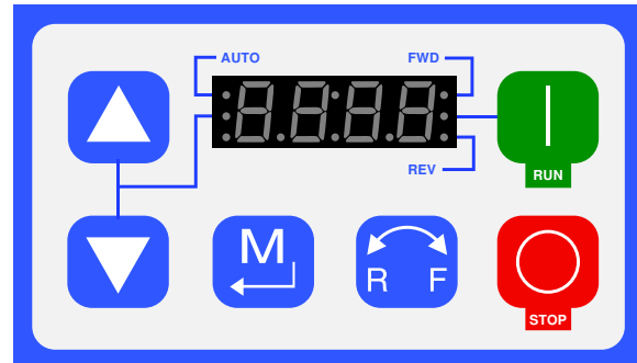
Figure 7 VFD Control Panel
